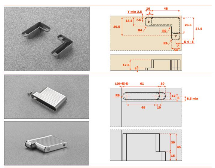
Formulas to determine the distance for the insertion of the sleeves for arm.
