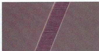
Tape-On-Top Splice: ONLY for applications with either platen or steel contact wheel. The abrasive grain is removed and the tape is applied to the grain side of the belt. This provides a bi-directional splice that is thinner at the splice than the rest of the belt.
