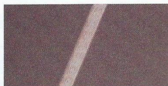
Lap Splice Top Skived: may only be run in one direction. Best for shape sanding with "J" Wgt. cloth belts.
